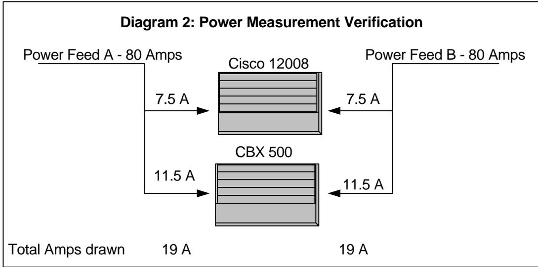
Using the **Sentry's Load Sense** option, the amount of power being used at each DC circuit is measured in a real-time manner. The result of real-time power measurement allows more equipment to be added on existing power resources (Diagram 3):
