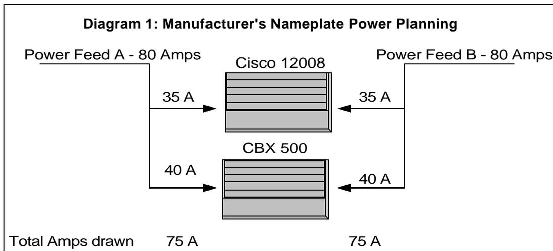
Using the manufacturer's nameplate specification for power consumption (Diagram 1) would indicate that the available power resource has been maximized.
