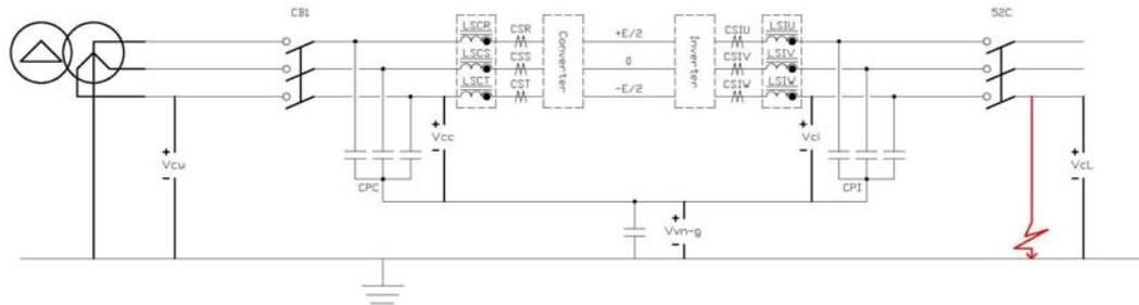
A Phase to Ground fault when the upstream transformer is grounded will produce high amounts of current in the inverter phases and will be detected by the UPS logic.
