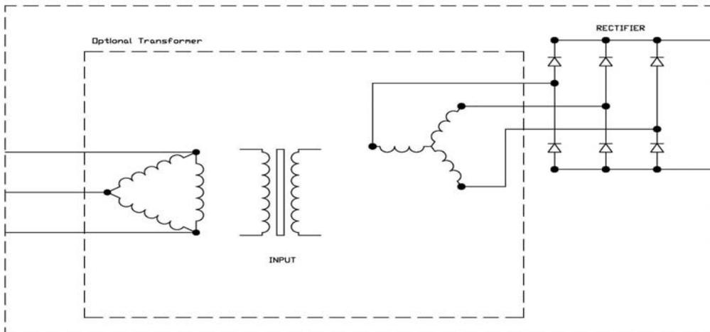
**Figure 3: Diode Bridge rectifier with optional transformer**
