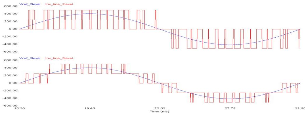
**Figure 7: IGBT Switching 2-level (top) and 3-level (Bottom)**
