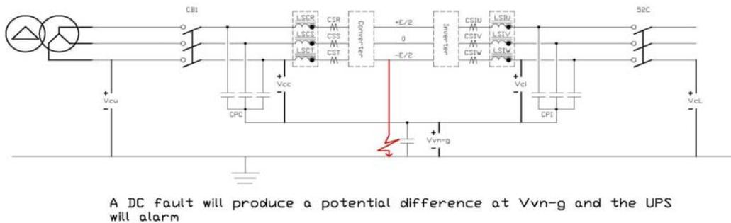
**Figure 13: DC Ground Fault**
