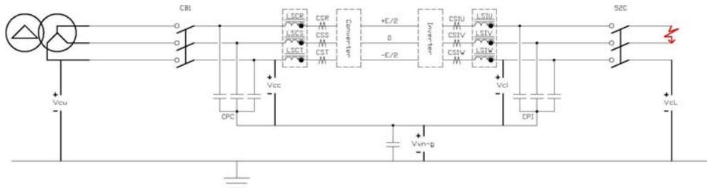
A Phase to Phase fault will produce high amounts of current in the inverter phases and will be detected by the UPS logic.
