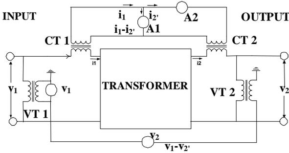
Connection Diagram for a Single-Phase Transformer
