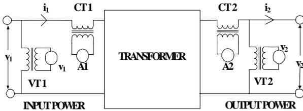
Connection Diagram for a Single-Phase Transformer
