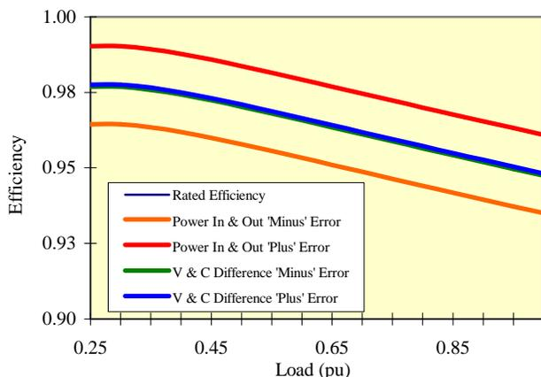
Efficiency Measurement Error
