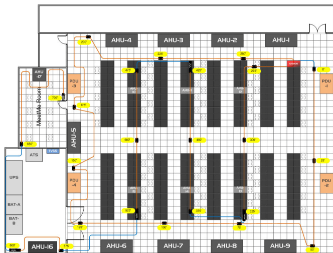
Uploaded reference map can be configured to display the location of the leak
